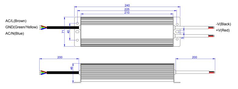
Cable Model of input: VDE H03V<sup>2</sup>V-F 3×0.75mm Cable Model of output: VDE H03V<sup>2</sup>V-F 2×0.75mm
